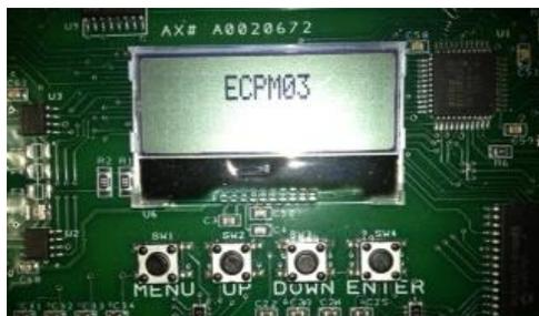
The ECPM03 board allows the user to configure a broad range of options associated with the functionality of the system through the setup menus on its LCD as shown above. Below the ECPM03 LCD are 4 buttons for navigation: MENU, UP, DOWN, ENTER.
